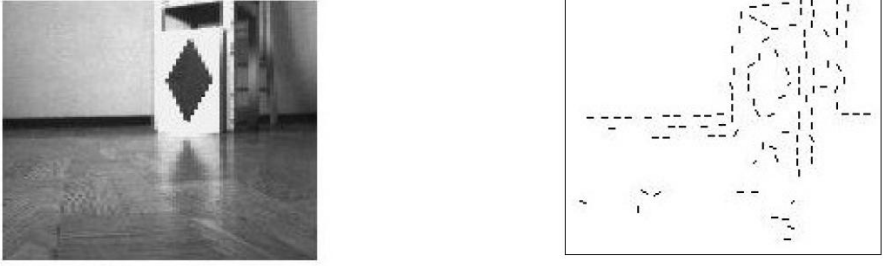
Fig. 2. An exemplary input image (left) and the corresponding visual primitives (right)
